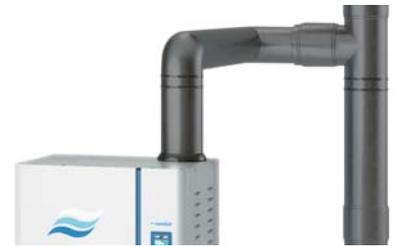
The lower flue gas temperature, created by the condensing technology, allows the use of plastic rather than stainless steel flues. This reduces the installation cost when compared to non-condensing gas-fired humidifiers.
