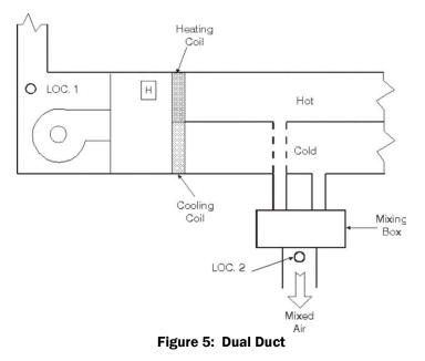
This system usually requires two steam distributors. The primary load (LOC.1) will go upstream of the fan. The humidistat is located after the fan and before the hot and cold decks. The secondary load (LOC. 2) will go downstream to the mixing boxes and will be controlled by a humidistat in the space. Please consult your Condair agent if absorption distance is a problem. High limit humidistat is recommended in the mixed air duct.
