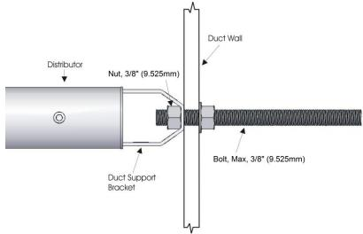
Figure 11: Duct Support Bracket Flush with Duct Wall
