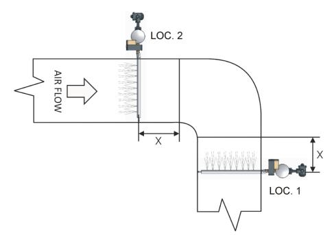
Note: If not calculated, dimension "X" is minimum 6'(1.82m) before or after bend or transition. See up flow effect on page 6 for calculation.
