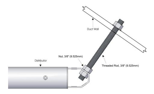
Figure 13: Duct Support Bracket with Angled Duct Wall
